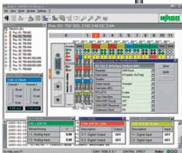
Configuration via WAGO-I/O-CHECK for example
