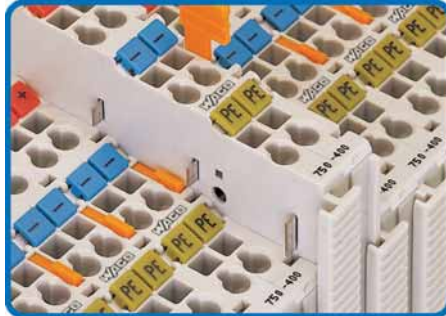
Safe, automatic connection by tinned, self-cleaning slide contact, ground (earth) contact makes first and breaks last (Series 750 and 753)
