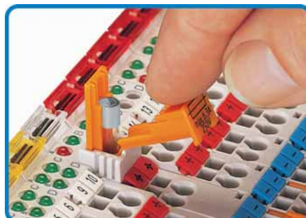
Function at locked position 2: Easy fuse replacement via hinged cover. Use UL-recognized fuses only!
